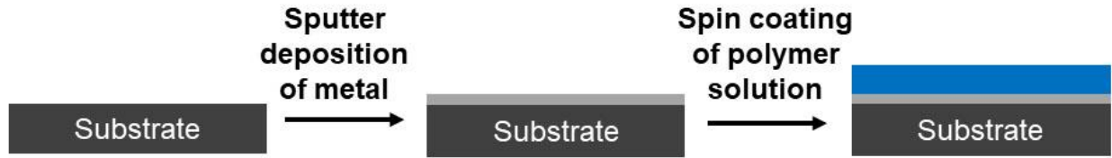
Figure 3.2. Schematic illustration of the preparation of the thin films of polymer on metal-coated substrates.
