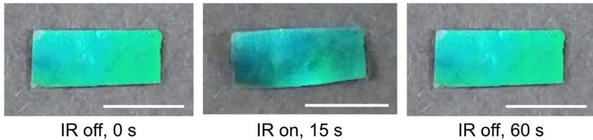
Figure 2.19. Photographs (top view) of reversible twisting and untwisting of the laminated film in response to global IR irradiation. The top-view photographs are taken at the fixed angle that is perpendicular to the substrate. Scale bar: 5 mm.
